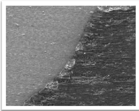
Weld/Base Interface @ 100X
